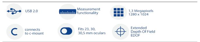
The large field of view allows you to capture more details with one image. You can replace one of the eyepieces of the microscope by the Dino-Eye camera which has a diameter of 23mm, or you can use one of the provided adapters of 30mm or 30,5mm to make it fit.
