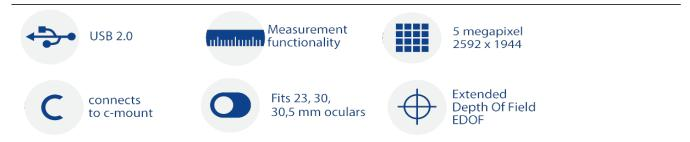
The large field of view allows you to capture more details with one image. You can replace one of the eyepieces of the microscope by the Dino-Eye camera which has a diameter of 23mm, or you can use one of the provided adapters of 30mm or 30,5mm to make it fit.
