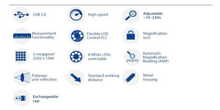
The Dino-Lite AM73515MZT is a USB 3.0 model with a magnification range of 10x - 220x and a standard working distance of up to 6 cm. This model is member of the Dino-Lite Edge family with the latest, cutting-edge optics, an unmatched 5 megapixel sensor and several special features such as Automatic Magnification Reading (AMR), Flexible LED Control (FLC), built-in polarization filter, full metal body, extensive measurement functions, calibration, exchangeable front caps and more.
