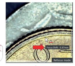
This cursor [ $\triangleright_A$ ] indicates that refocus mode is active and that the focus can be readjusted. A positive focus shift refers to a plane below the reference plane.
