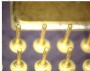
CPU pins without EDOF
